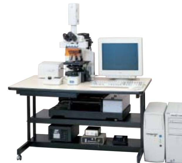
C1 system configured with E600 microscope
